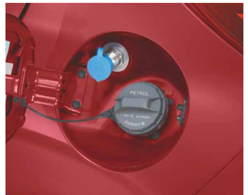
Convenient CNG filling with fast refuelling nozzle (near petrol filling area)
